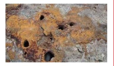
during fuel deliveries, acetic acid is deposited throughout the UST system. This results in a cycle of wetting and drying of the equipment which concentrates the acetic acid on metallic equipment causing severe and rapid corrosion. Contamination may be occurring in pipelines, terminal systems, cargo tank compartments or manifold vent systems.
