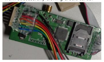
New skimmers are using chips, like the SIM900, a quad-band GSM/GPRS module with a very powerful single-chip processor as the backbone of the newest generation skimmers. Skimmers are not a new problem, but the technology that powers them has markedly improved over time. Previous incarnations were easy to spot with the naked eye, but newer versions are all but invisible.
